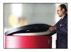
To lift the unit itself, first remove the thermoplastic cap on top and expose the transport eyebolts. Particularly for the tanks with steel sheet sleeve, care must be taken not to break the cap or deform the sheet when removing the cap.
