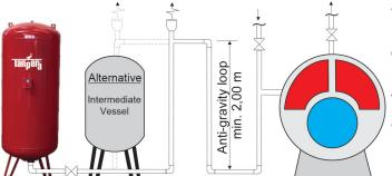
and above, the volume of water in the connection pipes of the tank must be at least as large as the expansion amount. If this is not possible (it is usually not possible to achieve this in large systems), to prevent hot water from reaching the bladder as much as possible, it is advisable to connect an intermediate vessel at the appropriate capacity into the pipework between the boiler and the
